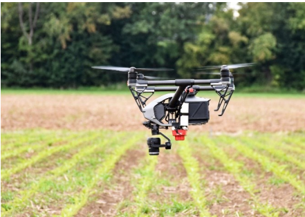
Aerial robot with different sensors
